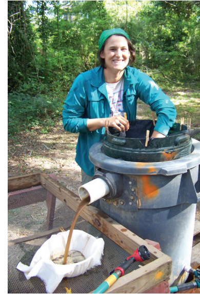
Figure 8. Katie Leslie processes soil samples from 3MN298 features using water flotation method at the Survey's HSU Research Station (photograph by Mary Beth Trubitt). The "heavy fraction" was caught on 1.0 mm mesh screen in the tank and the "light fraction" flowed out to be caught in the 0.25 mm mesh.
